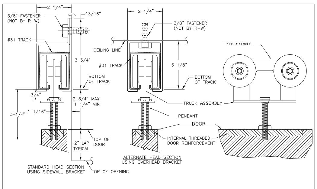
NOTE: SOME INSTALLATIONS MAY REQUIRE BRACKET SHIMS TO PROPERLY ALIGN THE TRACK.
